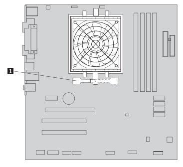
Figure 16. Removing the heat sink and fan assembly
